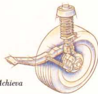
Achieva suspensions with MacPherson front struts and rear coil springs are tuned to provide a smooth, even and controlled ride.
